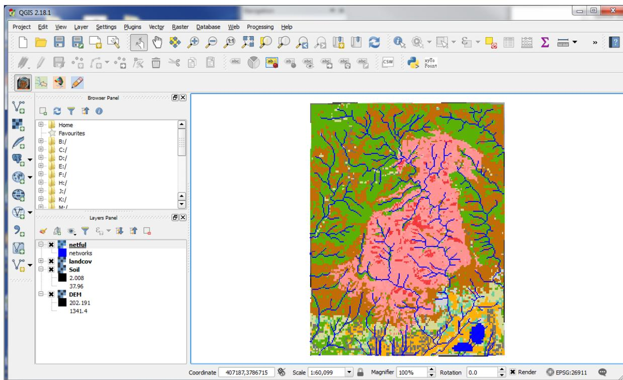
4. The next step is to select a watershed outlet and delineate the watershed using the select watershed button. Click on the button and then click on the map. This can be repeated multiple times to obtain desired watershed.
