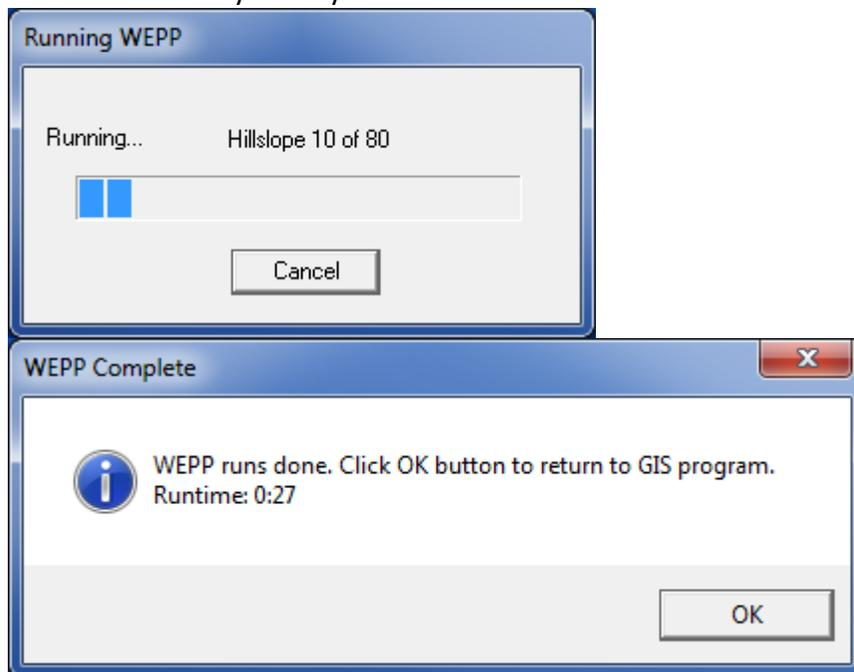
12. The output layer is stretched map showing hillslope sediment yield in Mg/ha. Within your QWEPP project a Results folder is created containing model outputs for your run using the name you supplied in step 6.
